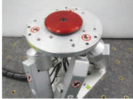
To avoid damages, the HXP50-MECA Hexapod is delivered with a locking system that includes a center rod and a clamping wheel.
